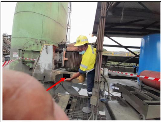
Figure 1: Re-enactment of how IP came in contact with moving pump belts.
